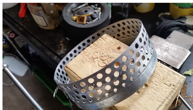
Flattened strip bent to shape ready to trial a diameter
